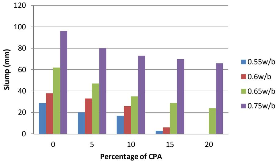
Figure 3: Slump values of CPA concrete at different water binder ratio
