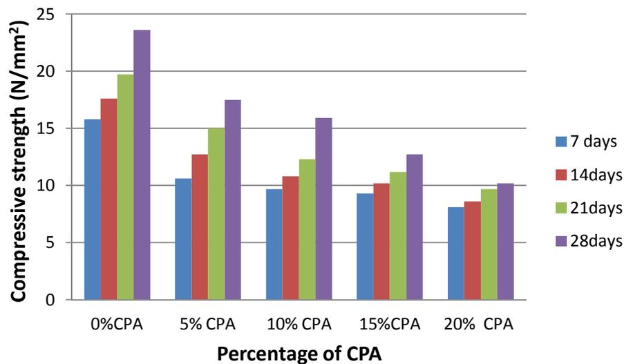
Figure 5: Compressive strength of CPA concrete at different curing days
