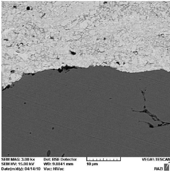
Fig.3: SEM micrograph of substrate-coating interface
