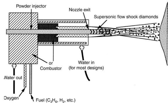
Fig. 1: High velocity oxy-Fuel thermal spraying
