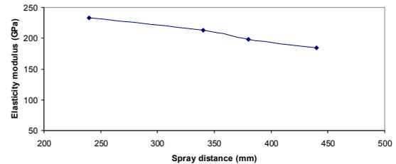
Fig.5: Measured elasticity modulus of WC-12Co in N=200g in different spray distance
