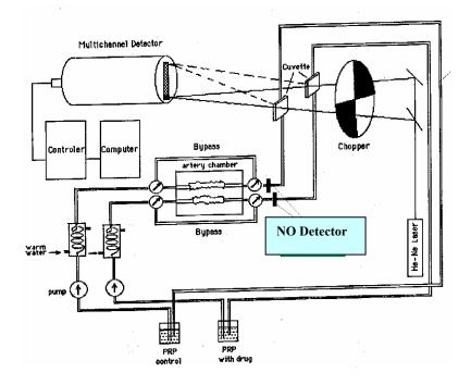
Figure 2. Dual Organ Chamber and Laser-light Scattering System
