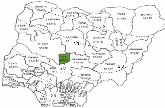
Figure 2. Distribution of annual average wind speed (m/s) at 10m height in Nigeria (Iloeje, 2004)
