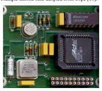
Fig. 4. The electronic board of the sample missile fuze adopted from Cope [10].
