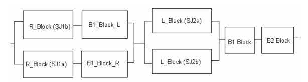
Fig. 5. The reliability block diagram of fuze electronics
