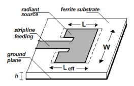
Figure 1. Geometry of microstrip rectangular patch antenna.
