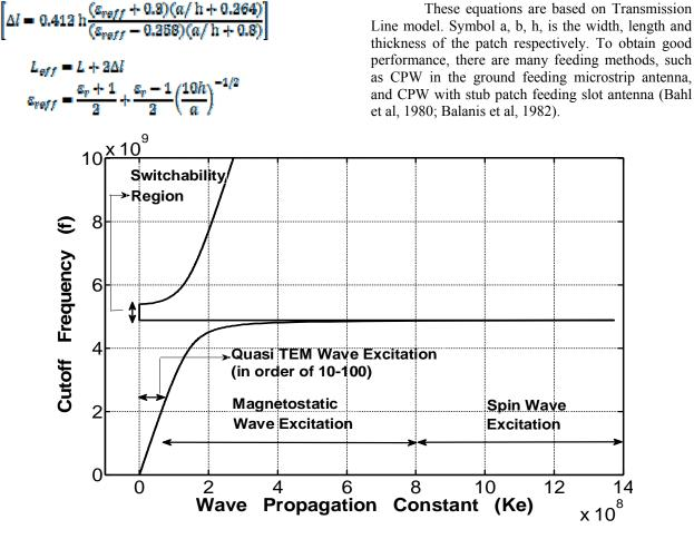
Figure 2. Dispersion curve (f vs. K) for plane wave propagation perpendicular to biasing field.
