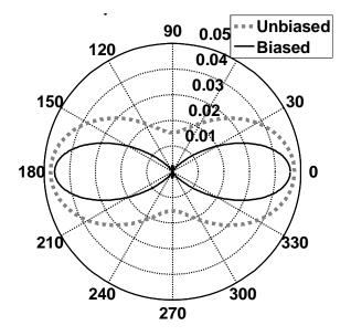
Figure 3. Comparison of E-plane pattern of rectangular patch microstrip antenna with RHCP for unbiased case and biased case.
