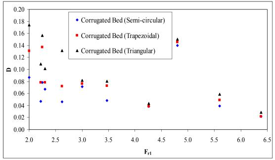
Figure 5. Relation between depth dimensionless index, D and  $F_{r1}$
