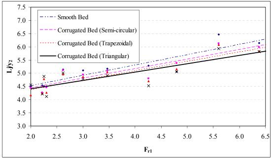
Figure 6. Relation between the ratio of  $L_i/y_2$  and  $F_{r1}$
