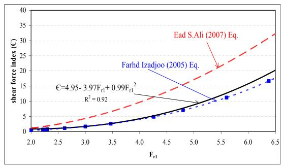
Figure 9. Shear force index for hydraulic jump over corrugated beds
