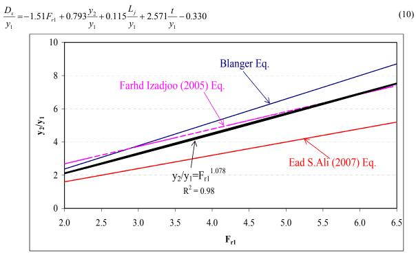
Figure 4. Relation between  $y_2/y_1$  and  $F_{r1}$  for classical jumps and jumps over corrugated beds
