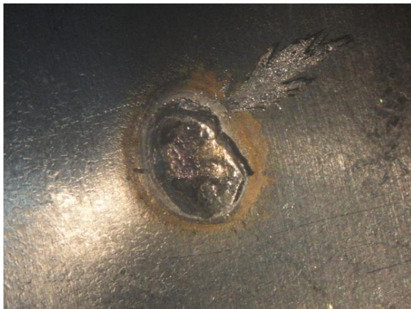
Fig. 6 Molten metal explosion from nugget.
