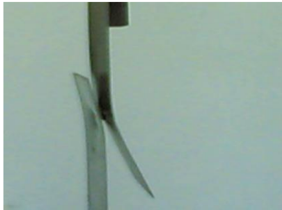
Fig. 3 Tensile test for the spot welded specimens.
