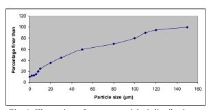
Fig. 1. Illustration of cement particles' distribution.
