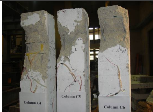
Fig. (9) crack pattern and the shape of failure of c4 , c5 , c6
