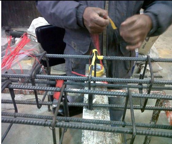
Fig. (3) Fixing electrical strain gages
