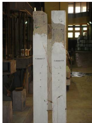
Fig. (10) crack pattern and the shape of failure of c7 , c8
