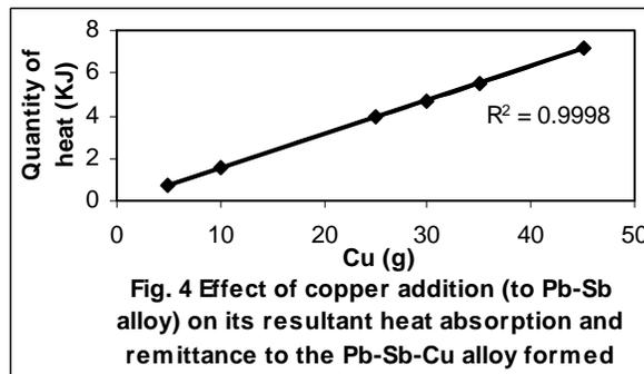
temperature incurred. An evaluation of the correlation coefficient, R between the Cu added to the base alloy (Pb-Sb alloy) and heat absorbed and remitted to the formed Pb-Sb-Cu alloy (as in Fig.4) using the equation;
