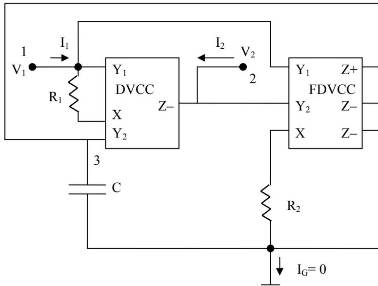
Figure5 A modified floating inductor using DVCC and FDVCC [18]
