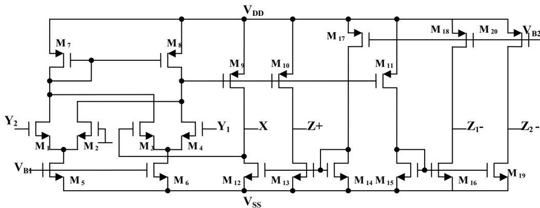
Figure 9 CMOS circuit of the floating DVCC [21]
