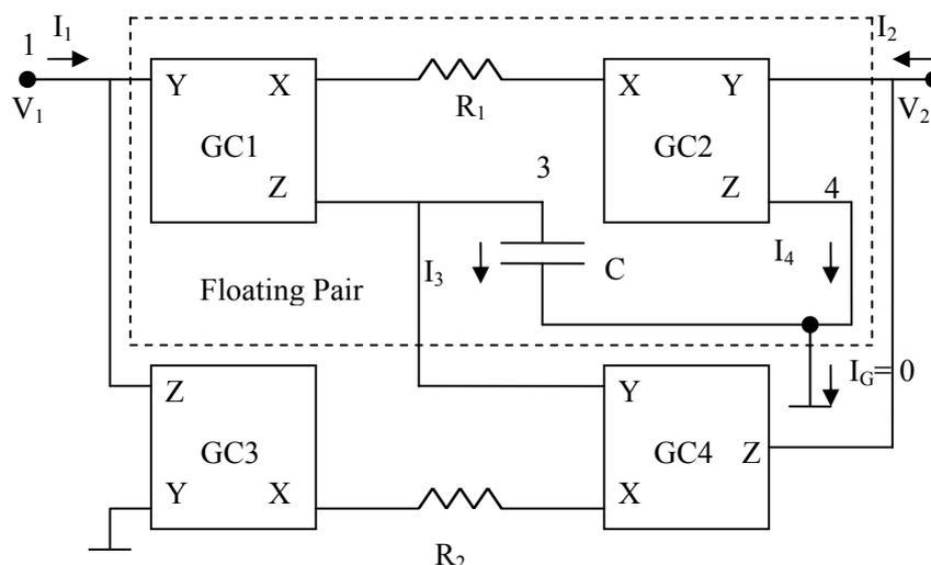
Figure 2. A floating inductor using four generalized conveyer
