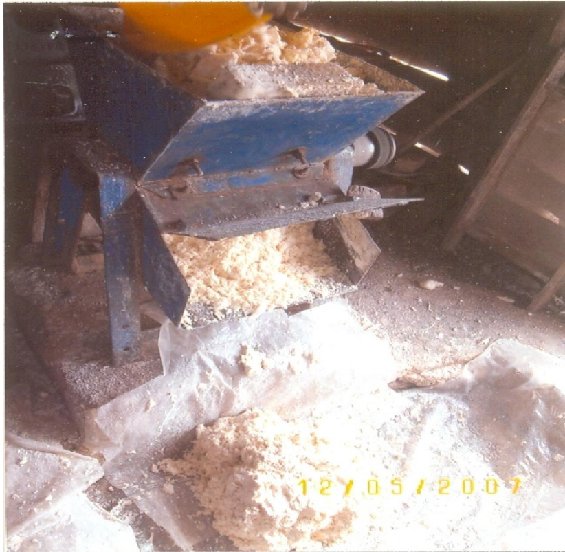
Figure 5: This shows the process of grating cassava white pulp using a grinding machine
