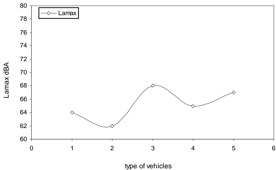
Figure 3. Effect of vehicle type on its L Amax of pass-by noise emission at 50Km/hpur speed
