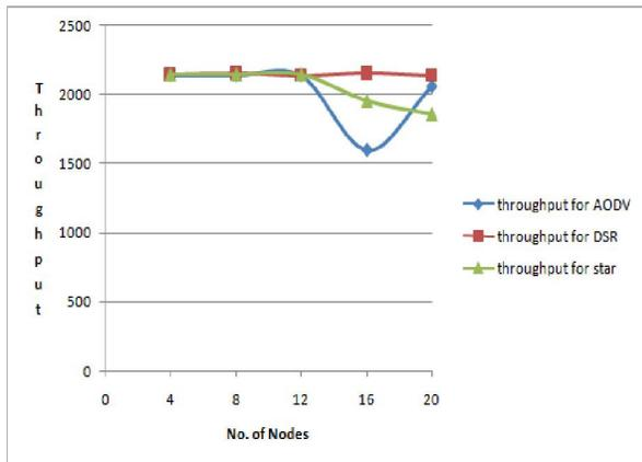
Fig.1 Throughput vs. No. of Nodes for packet sizes 256 bytes
