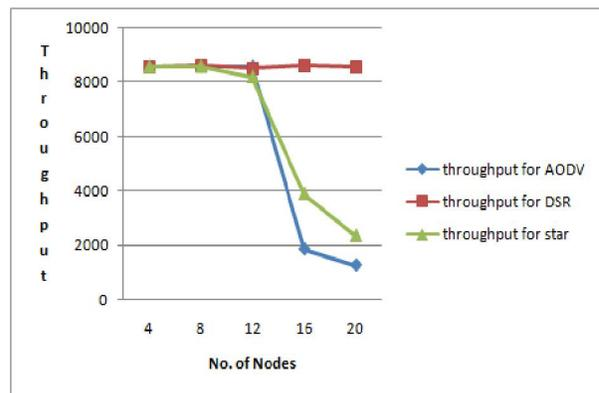
Fig. 3 Throughput Vs No. of Nodes for Packet sizes 1024 bytes
