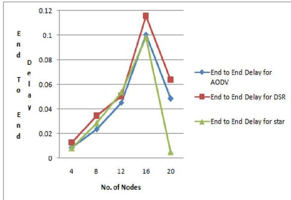
Fig. 5 End to End Delay Vs. No. of Nodes for Packet sizes 512 bytes.
