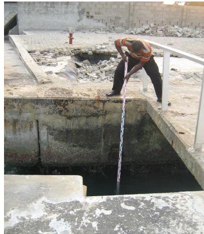
Fig.11: Tidal Lag observation using leveling staff
