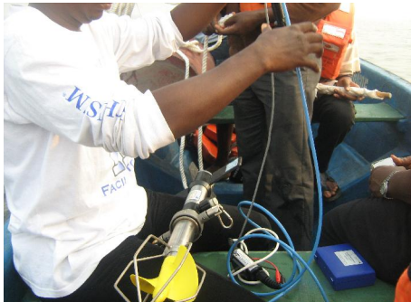
Fig. 3: Current meter fixing, ready for
