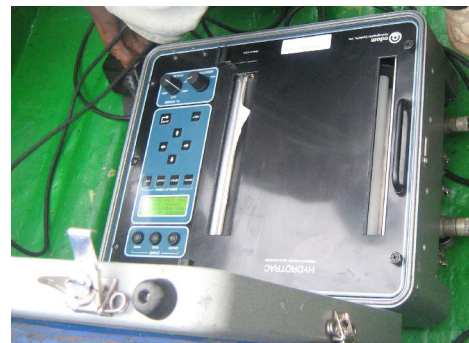
Fig. 7: Echo sounder instrument being
