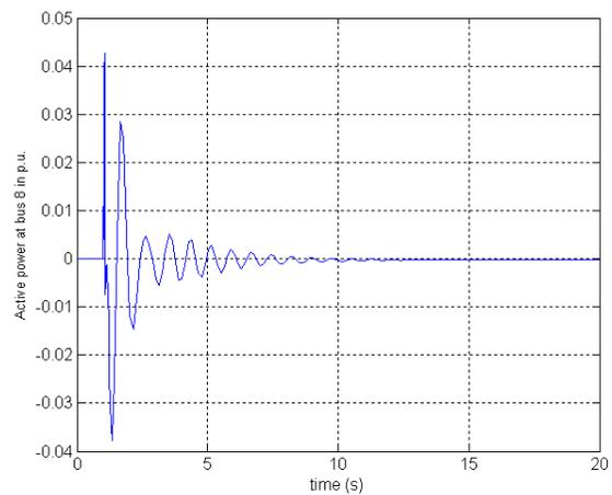
**Fig.13:** Active power at bus 8 due to line 5-6 outage at  $\lambda=1.6$  p.u. for system with (CNT)
