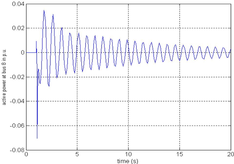
**Fig.9.** Active power at bus 8 due to line 5-6 outage at  $\lambda=1.6$  p.u.
