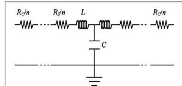
**Fig.2.** Equivalent RLC circuit diagram of the bundled (CNT) coaxial via scheme (long length with the assumption of ideal contacts)
