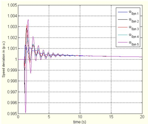
**Fig.11:** Generator speed oscillation due to line 5-6 outage at  $\lambda=1.6$  p.u. for system with (CNT)
