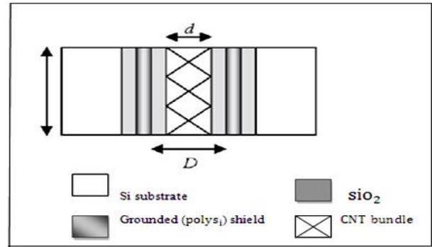
**Fig.1.** Cross-sectional view of the bundled CNT based coaxial
