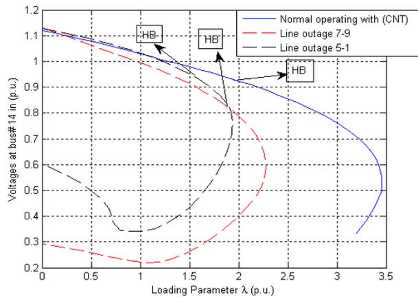
**Fig.10:** P-V curves at bus# 14 for emergencies and normal operating with (CNT)
