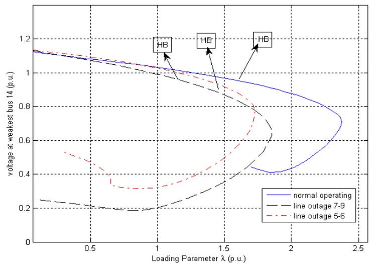
**Fig.6.** P-V curves at bus# 14 for two emergencies with base case
