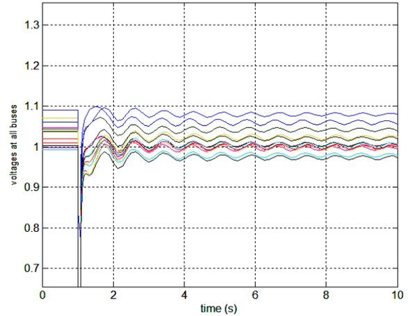
**Fig.8.** Voltages at all buses due to line 5-6 outage at  $\lambda=1.6$  p.u.
