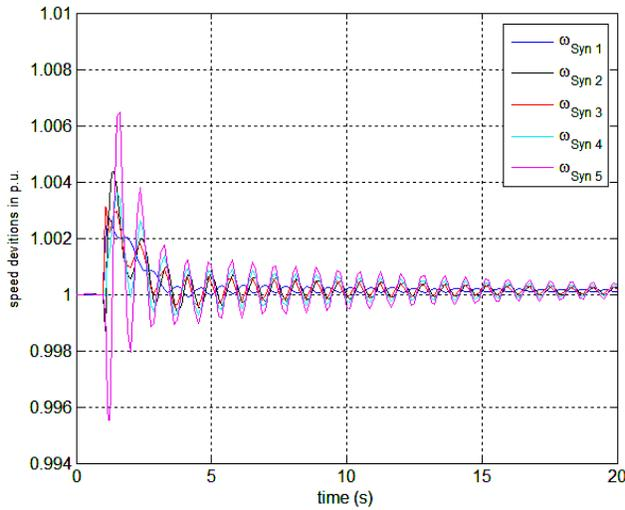
**Fig.7.** Generator speed oscillation due to line 5-6 outage at  $\lambda=1.6$  p.u.
