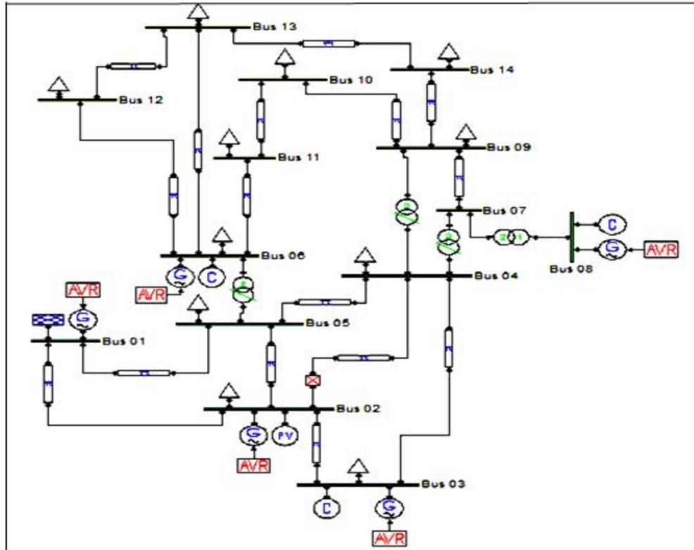
**Fig.5.** Single line diagram of IEEE 14 bus test
