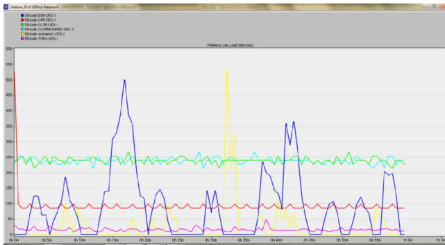
Fig. 7 Time Average in WLAN Load in bit/sec for MANET 50 Nodes
