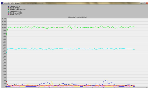
Figure 8 WLAN THROUGHPUT IN BIT/SEC FOR MANET75 NODES
