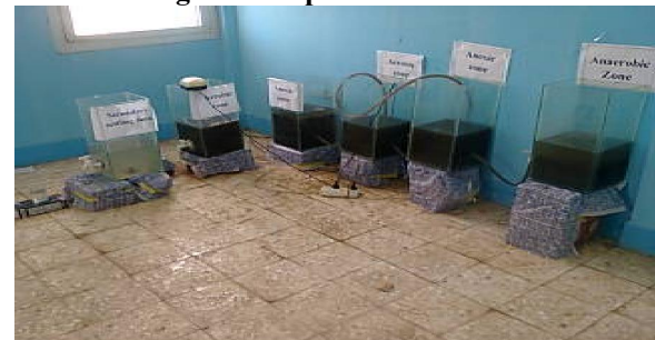
Figure 4: 5-Stage Bardenpho Process
