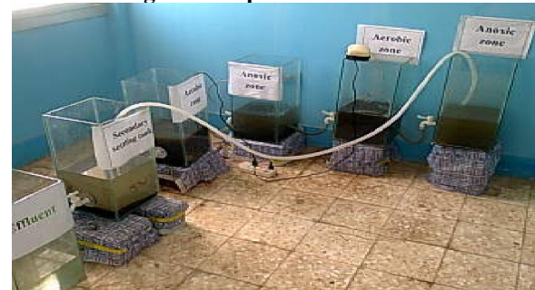
Figure 3: 4-Stage Bardenpho Process
