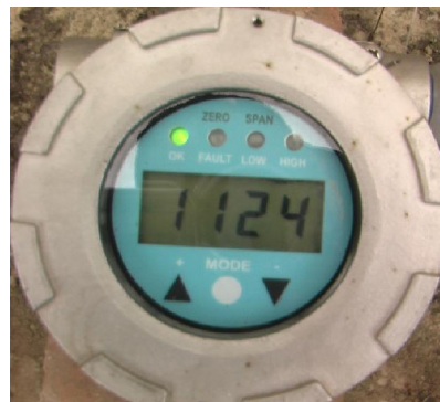
Figure 10. Measurement of carbon dioxide emissions device
