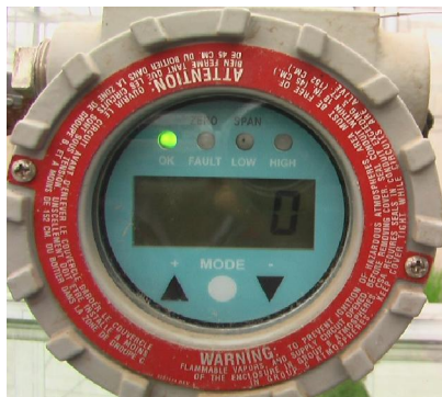
Figure 11. Measurement of nitric oxide emissions device (mono nitrogen oxide)
