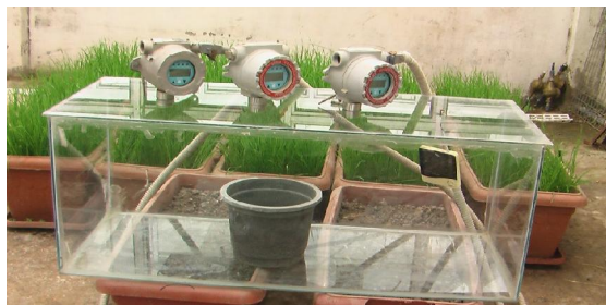
Figure 8. Shows the experimental unit, and measurement devices of CO 2 , NO and N 2 O it installed on the cover and the measurement of temperature and humidity device installed inside it and also pot content the soil placed inside
