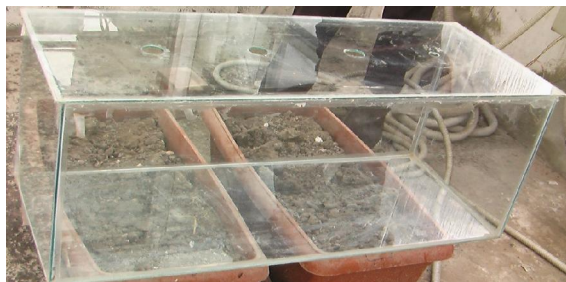
Figure 6. Shows the experimental unit (Glass Chamber) and the holes necessary to install the devices in the cover
