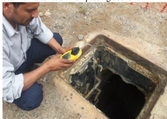
Picture (2) odor measurements at the MH.
