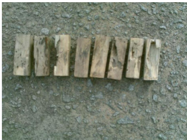
Fig. 4: Degradation of 20 mL treatment test blocks by termites after 3 months of exposure
