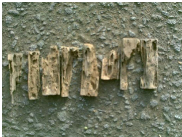
Fig. 3: Degradation of control samples by termites after 3 months of exposure
