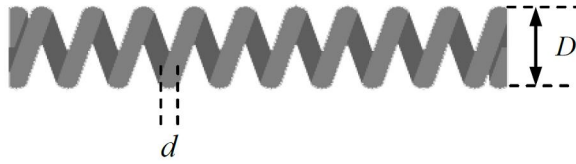
Figure 2. Geometry of single coiled linear tungsten filament.
