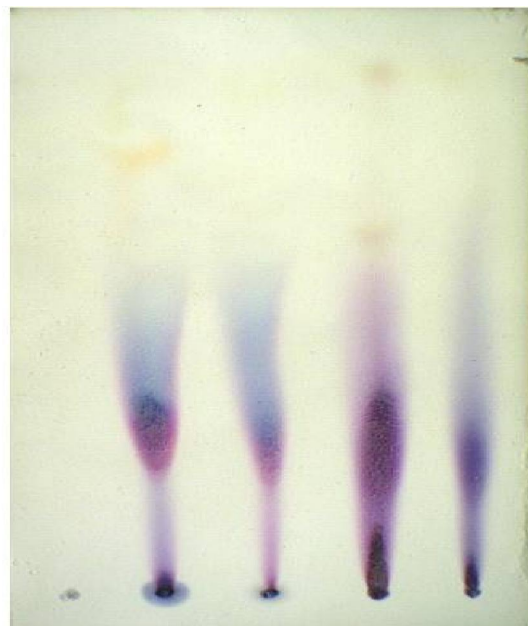
Fig (2) chromatogram of different brands ink (UV) at 254nm
