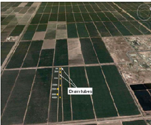
Figure 2. Aerial photo piezometers pipes placed between two drain pipes
