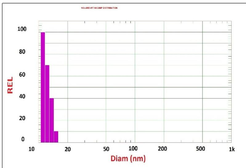
Mean Diameter = 11.5 nm Fit Error = 76.434 Residual = 91.132
