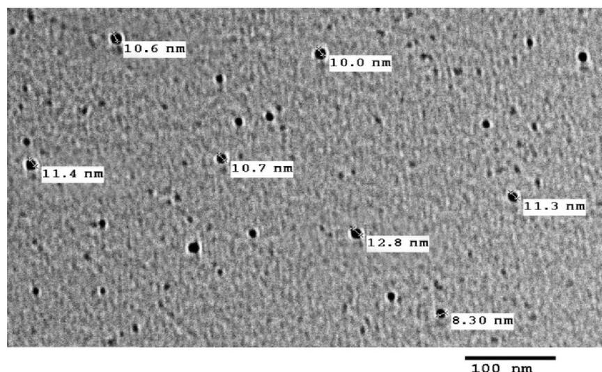
**Figure 6. Transmission electron microscopy (TEM) image of silver nanoparticles produced by *S. marcescens* isolate WSE****Fourier transform infrared spectroscopy (FTIR) spectral analysis**
