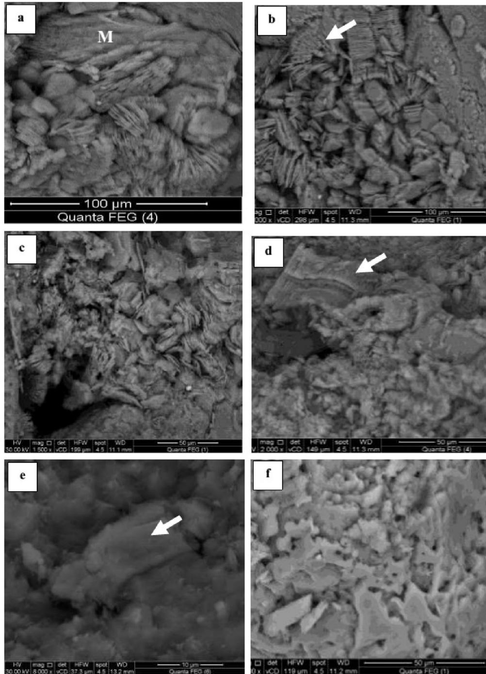
**Figure 9:** SEM images show a) neomorphosing detrital muscovite (M); b) some stacks joined together to compose a fan-shaped unit (arrow); c) the "shaggy" appearance of kaolinite books; d) altered feldspar grain to kaolinite. Its edges and surfaces of these stacks or books are irregular (arrow) and e) edges and surfaces of kaolinite stacks or books sometimes much smoother (arrow); f) quartz overgrowth on quartz grains.
