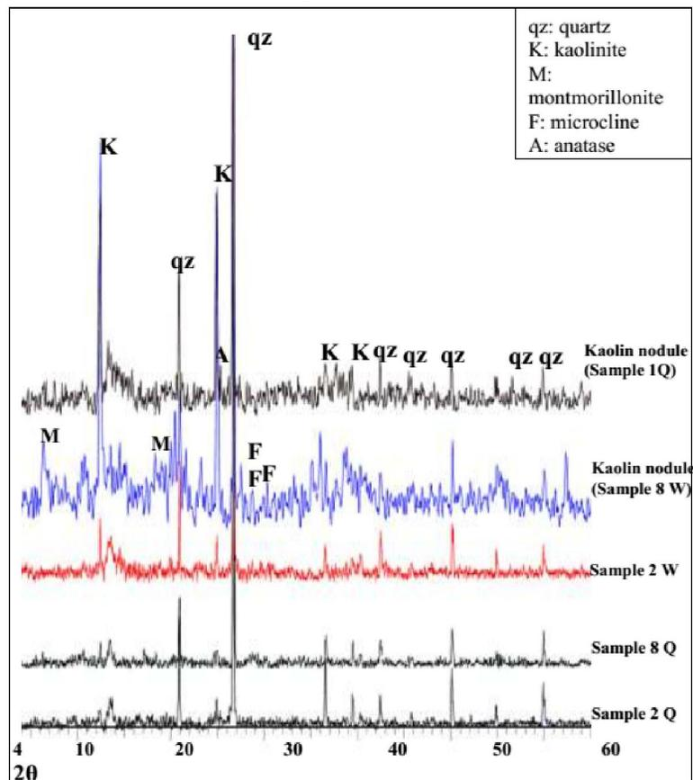
**Figure 7:** XRD patterns of some studied sandstones and kaolinitic nodules samples in both Wadi Qena (Q) and Wadi El-Dakhel (W) sections.
