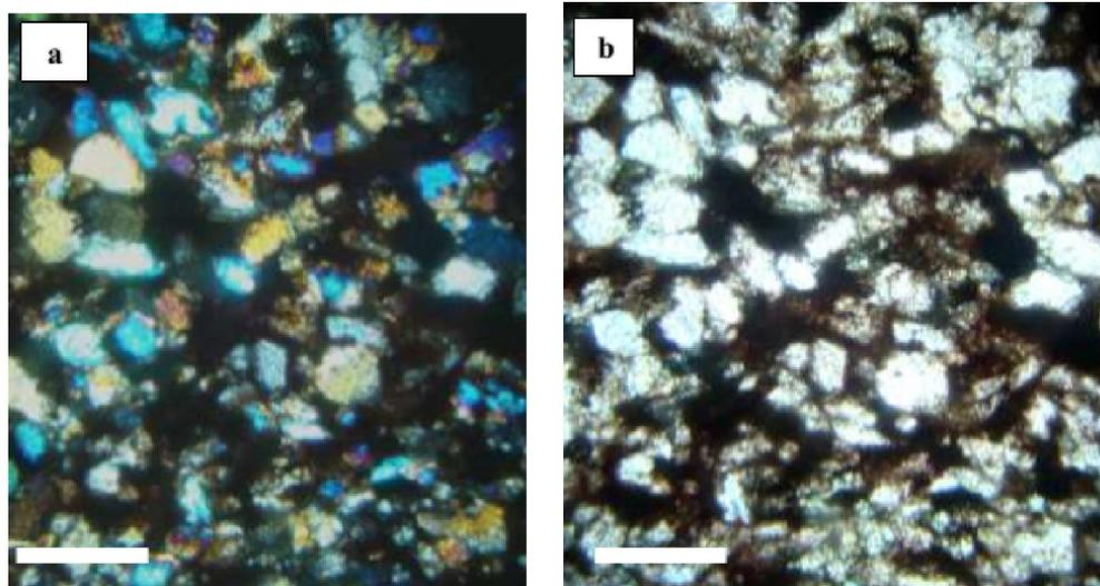
**Figure 5:** Photomicrographs show the ferruginous quartz arenite; a) under polarizing microscope; and b) under ordinary light. Bare scale = 0.5mm.
