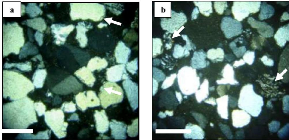
**Figure 4:** Photomicrographic views of quartz arenite sandstone of Naqus Fm. (a) Some quartz grains are encrusted by silica overgrowth (arrow). (b) Quartz arenite with a partial dissolution of white mica (arrows). Bare scale = 0.5mm.
