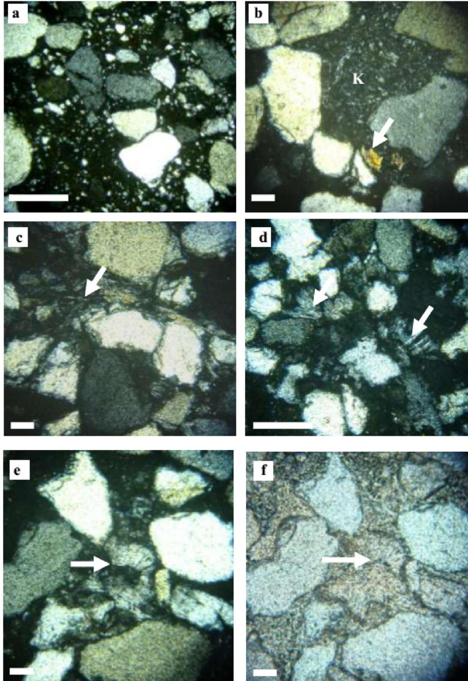
**Figure 6:** Photomicrographs show the quartz greywacke sandstone type; a) the scattered matrix in quartz wacke; b) authigenic kaolin (K) and muscovite grains (arrow); c) muscovite grain (arrow) that partially altered into clay matrix; d) vermicular stacks of sericite (?) as a result of partially dissolved mica grains (arrows); e) authigenic clay matrix (arrow); f) as (e) under ordinary light. Bare scale = 0.5mm.
