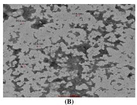
Fig. 4. HR-TEM image of CS NPs (A), and CS-HA nanocomposite (B).
