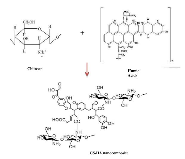
Fig.1: Structure of chitosan-humic nanocomposite (Cs-HA nanocmposite)
