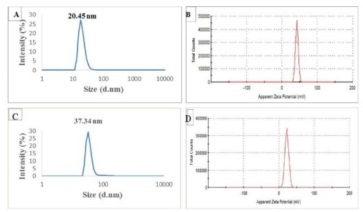
Fig. 3. DLS analysis of CS NPs, and CS-HA nanocomposite particle size (CS NPs (A), CS-HA nanocomposite (C), and Zeta potential CS NPs (B), CS-HA nanocomposite (D)
