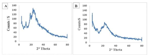
Fig. 2. X-ray powder diffraction patterns of chitosan nanoparticles (A) and chitosan- humic nanocomposite (B).
