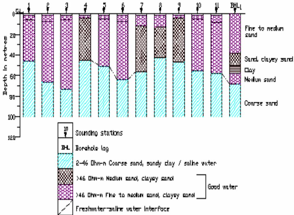
Fig 4: Representative sample of geoelectric sections correlated with borehole log 1
