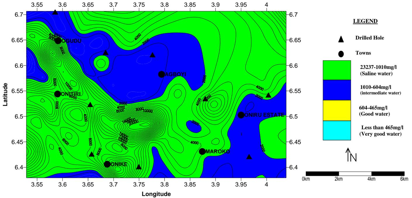
Fig 9: Morphology of subsurface TDS for layer III. Contour interval is 50mg/l
