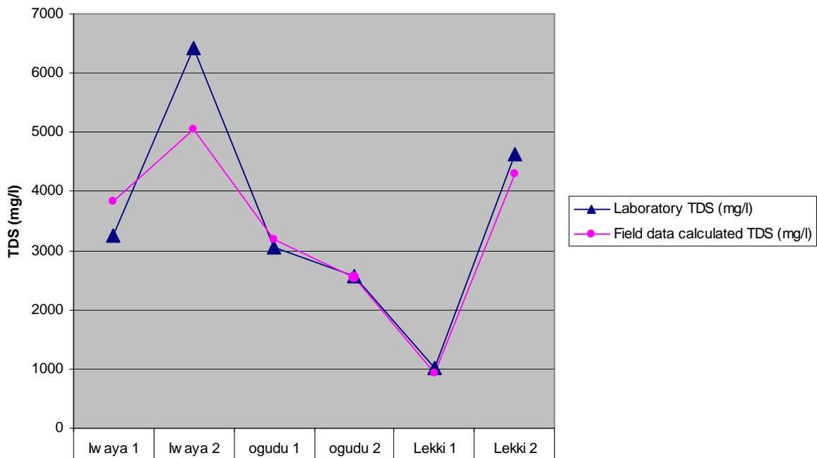
Fig 10: Comparison of Laboratory analysis of total dissolved solids (TDS) and TDS values inferred from resistivity data
