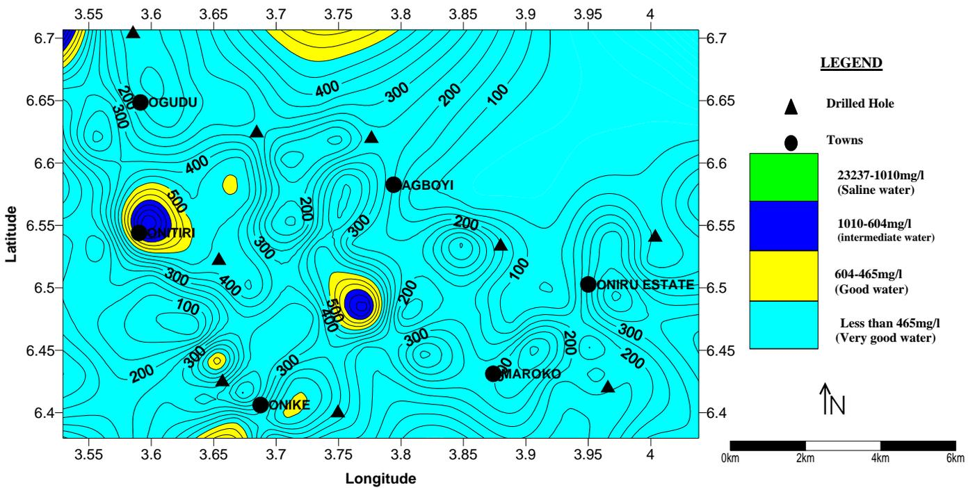
Fig 6: Morphology of subsurface TDS for layer I. Contour interval is 50mg/l.
