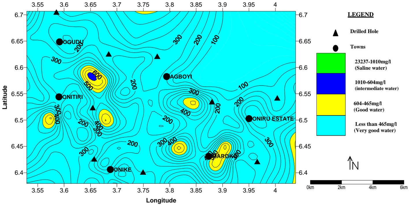
Fig 7: Morphology of subsurface TDS for layer II. Contour interval is 50mg/l
