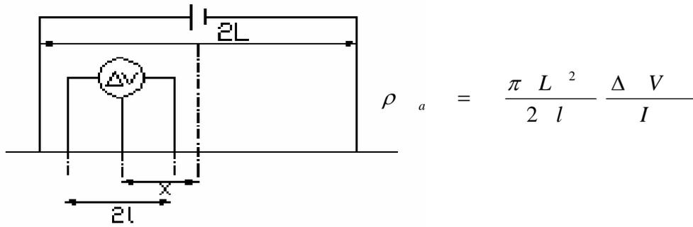
Fig 2: Schlumberger electrode array configuration
