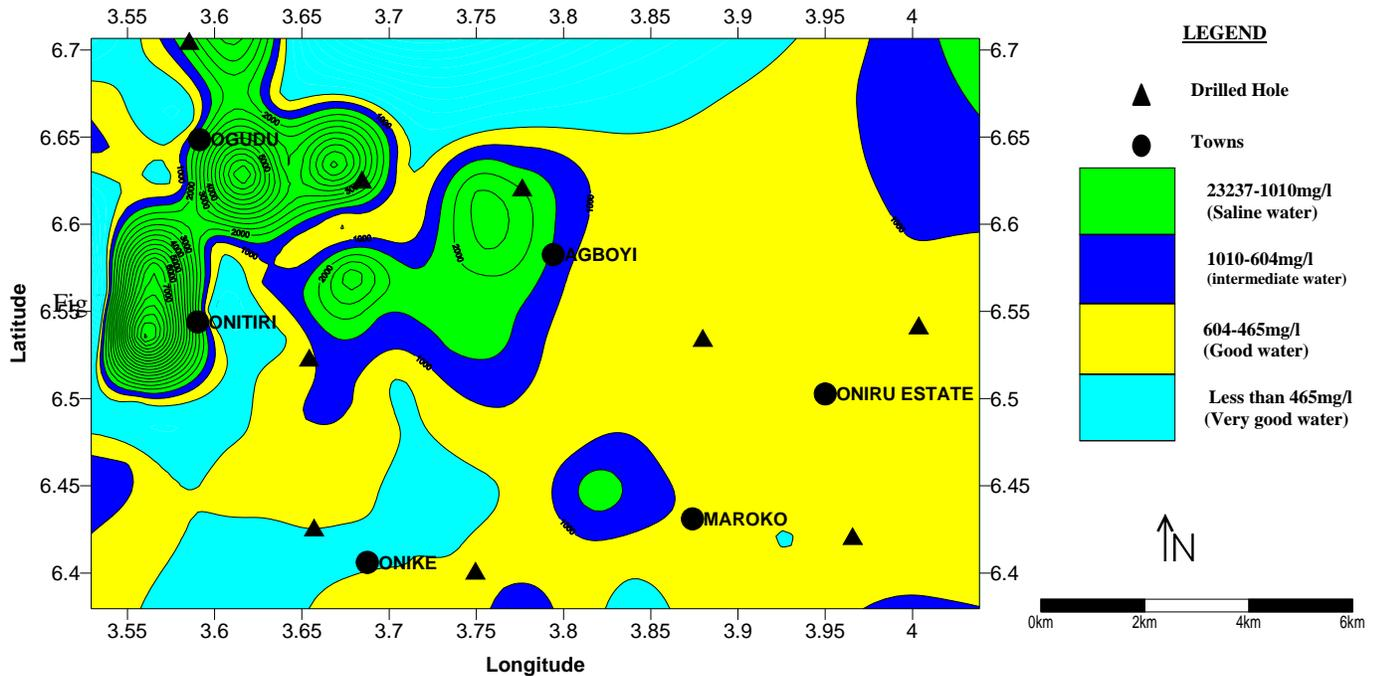
Fig 8: Morphology of subsurface TDS for layer III. Contour interval is 50 mg/l
