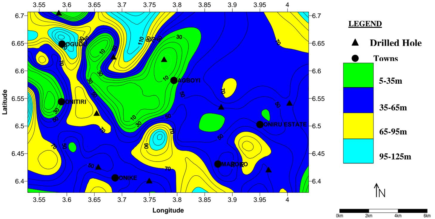
Fig 5: Depth to 0.5-0.022ds/m iso- conductivity surfaces. Contour interval is 10m. Average depth is 69m.
