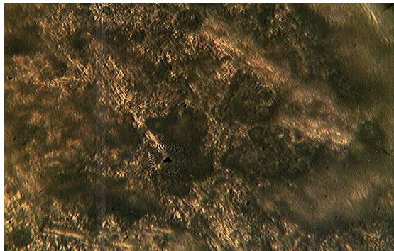
Fig.6-Microstructure of Pb-Sb matrix, 4.76%Cu x400
