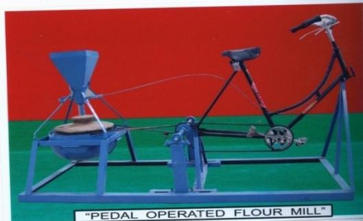
Figure3.pedal operated flour mill
