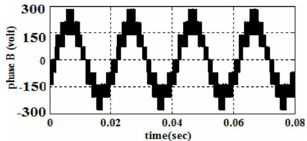
**Fig .6.b: The voltage wave form of phase B**
