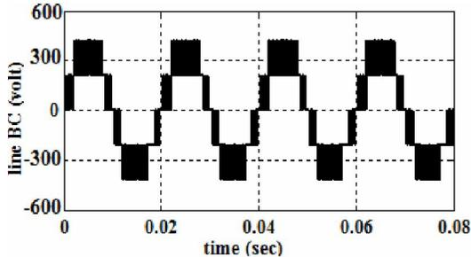
Fig .6.e: line voltages B C wave form
