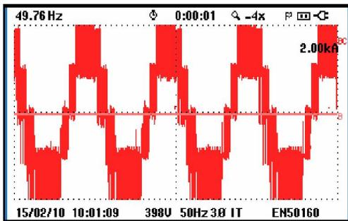
Fig.9.e: Experimental line voltage B&C wave form.
