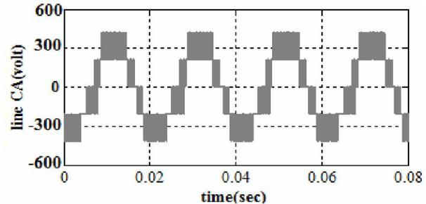
Fig .6.f: 1 line voltages CA voltage wave form
