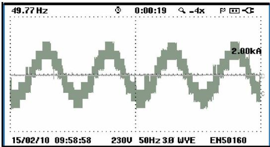
Fig .9.c: Experimental phase voltage C wave form
