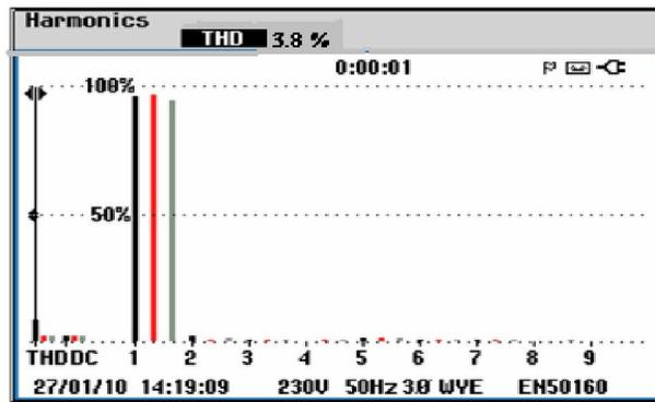
Fig. 10: Expeimetal THD Harmonics spectrum for three phase voltage.
