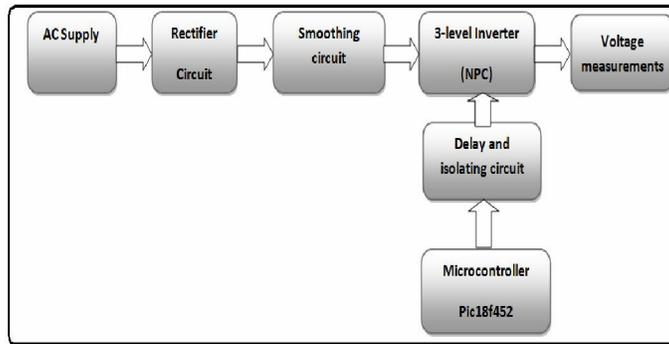
Fig .8: Schematic diagram of the experimental system
