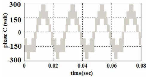
Fig .6.c: The voltage wave form of phase C
