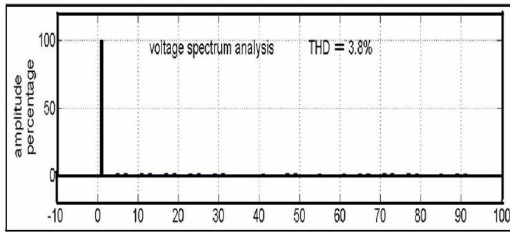
Fig .7: THD spectrum for phase voltage A
