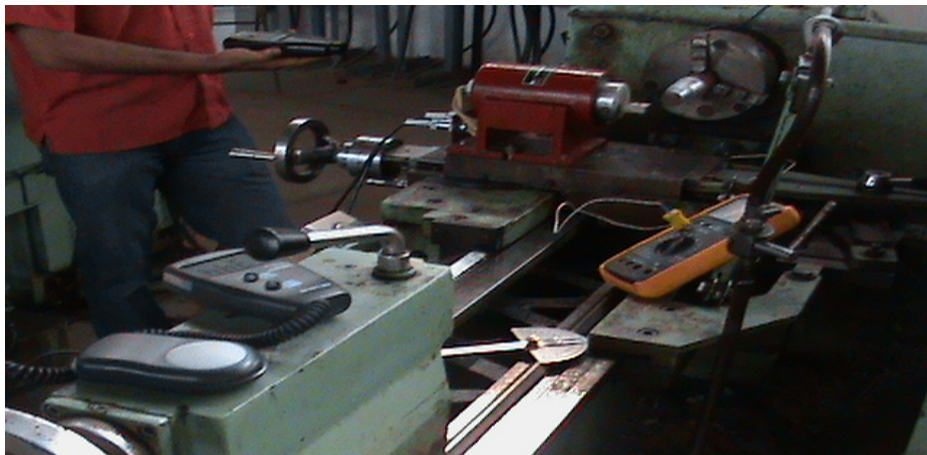
Figure 1. The experimental setup for turning Aluminum 6063
