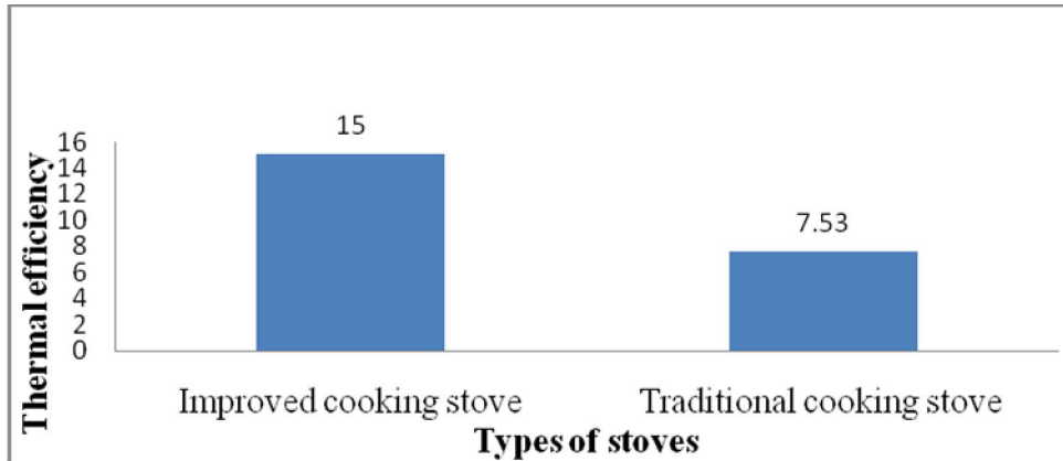
Figure 1: The thermal efficiency of used stoves
