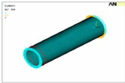
Figure 3 - shell modeling based on ANSYS Software
