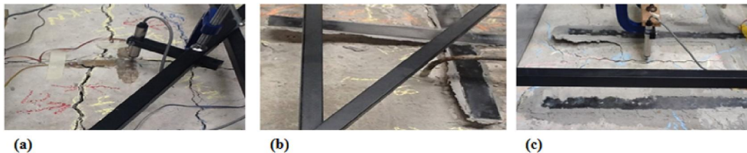
Fig. 3 – (a) Failure in Control Sample, (b) De-bonding in CFRP.500 Sample, (c) De-bonding in CFRP Plate in CFRP.BFRP Sample
