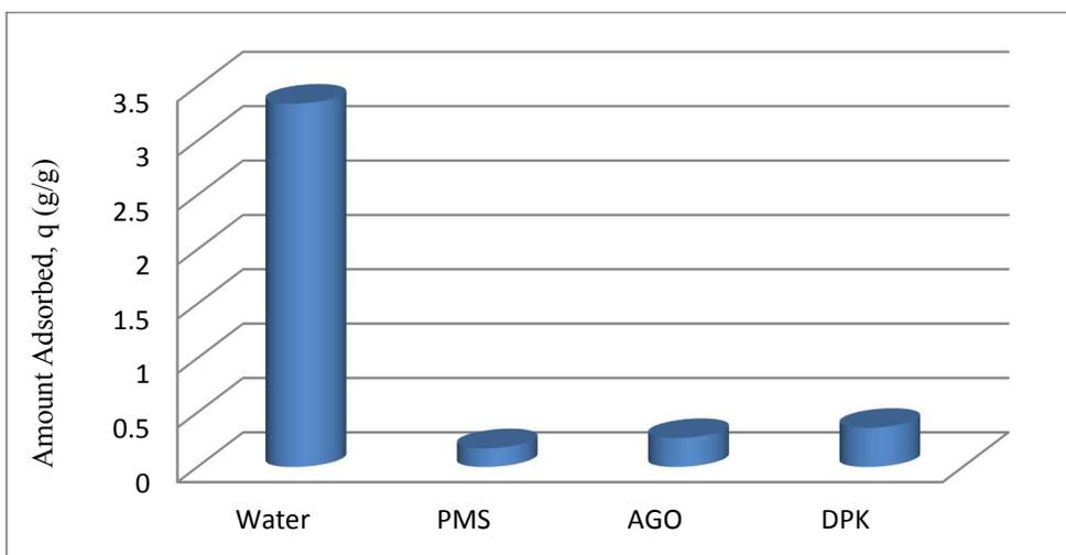
Figure 2. Adsorption capacity of water and organic solvents on sodium bentonite
