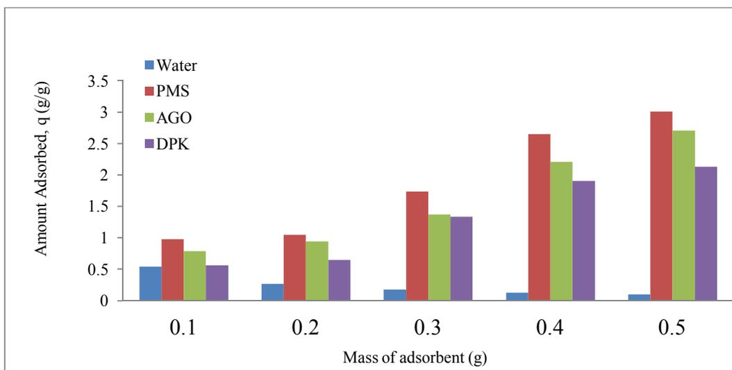
Figure 3. Adsorption capacity on TEAB-Modified bentonite
