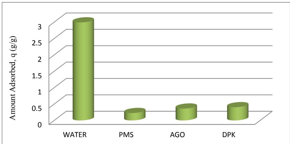
Figure 1. Adsorption capacity of water and organic solvents on unmodified calcium bentonite
