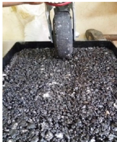
Figure (17) Slab under wheel load
