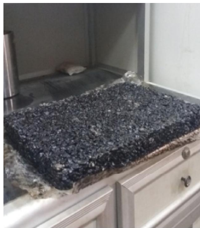
Figure (16) Compacted slab
