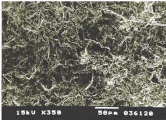
Fig. (3): SEM of acid etch metal surface treatment specimen group (II) before bonding (SEM photograph, original magnification 350×).
