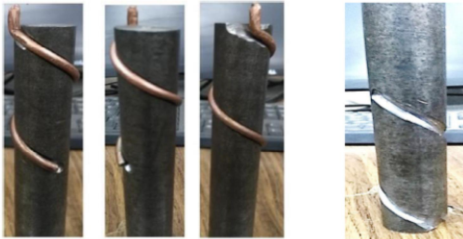
Fig. 4 Electrode bending on the mandrel Fig. 5 Mandrel after engraving process
