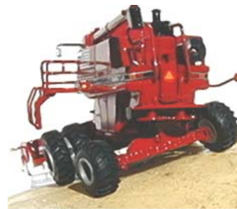
Figure 2. Adjusting the height of a combine by a hydrostatic drive
