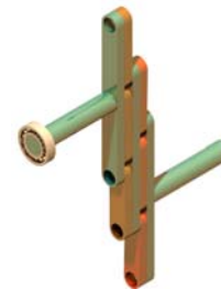
Figure 7. Dead point of balanced mechanism
