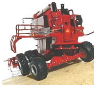
Figure. 2. Adjusting the height of a combine by a hydrostatic drive
