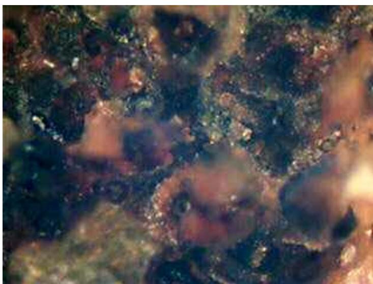
Plate 1: Micrograph of the uninhibited sample immersed after 336 hours of exposure. X 200
