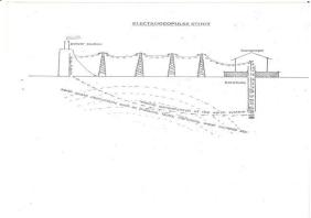
Observe the changes in the electric currents of the earth system 24 hours, 365 days. From a power station, the electricity is distributed to the far-off places. Normally the circuit of the power supply being completed through the earth system. Whenever if the
