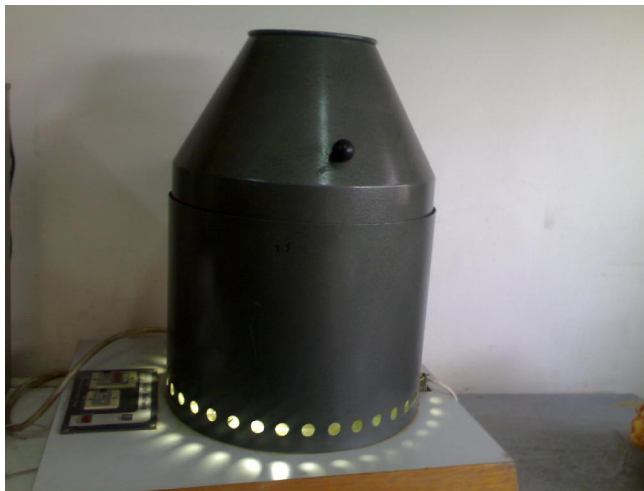
Fig. (1) : Batch microsol photoreactor light tester
