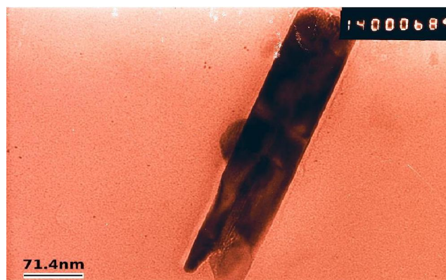
Figure 5: TEM image of CuO nanorods.
