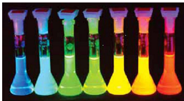
Fig 2: Fluorescence in different-sized CdSe quantum-dots
