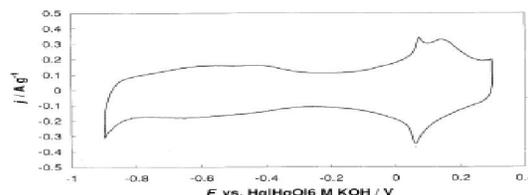
Fig 5 : CV taken at  $20 \text{ mV s}^{-1}$  of co precipitated  $\text{CaRuO}_3$
