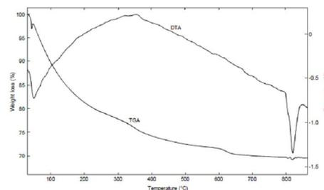
Fig. 1. TGA/DTA of n- $\text{CaRuO}_3$ .
