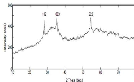
Figure 2: XRD of n- $\text{CaRuO}_3$ .
