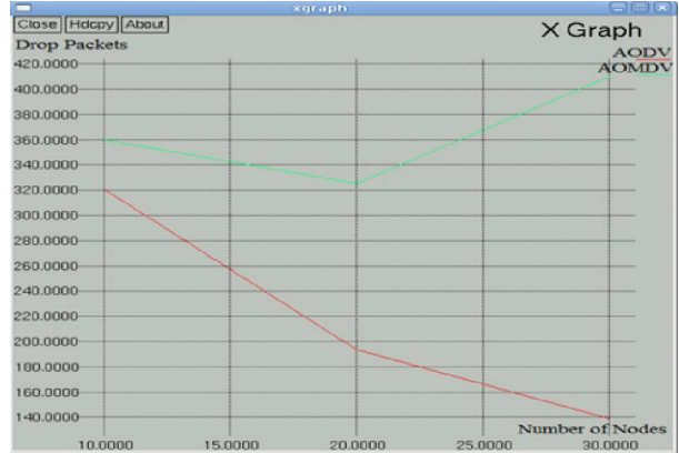
Figure (5): Comparison Dropped Packets for AODV & AOMDV with versus number of nodes (10, 20, 30).
