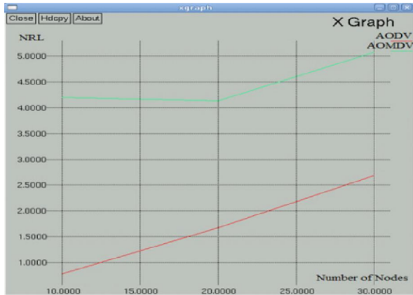
Figure (8): Comparison Normalize Routing Load (NRL) for AODV&AOMDV with versus number of nodes (10, 20, 30).
