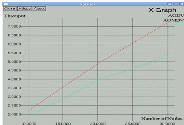
Figure(4): Comparison Throughput for AODV & AOMDV with versus number of nodes (10 , 20 , 30).
