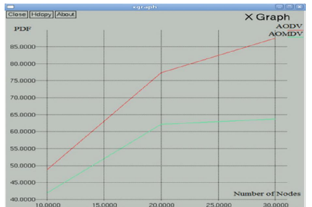
Figure (7): Comparison Packet Delivery Fraction (PDF) for AODV&AOMDV with versus number of nodes (10, 20, 30).
