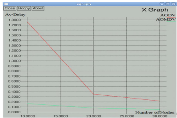
Figure (6): Comparison Average End-To-End Delay for AODV&AOMDV with versus number of nodes (10, 20, 30).
