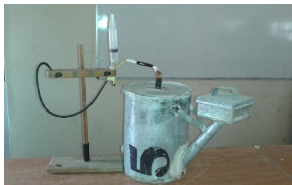
Figure 1: Laboratory scale (15L) biogas fermentor for assessment of gas yield
