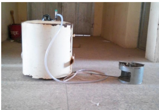
Figure 2: A 25 Liter biogas fermentor for flammability tests
